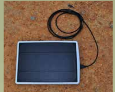
Solar panel for recharging
